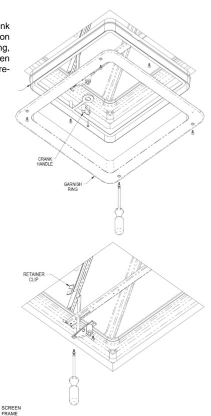
Remove the screws securing the lift operator and disengage the lift arm from the lid track. Some vent lids will employ a retainer clip over the lift arm rivet, remove and discard if present. Retain screws for reinstallation.
