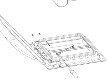
From inside the coach, engage slide/clip with T-bar on universal lid. Re-install lift operator with original screws.
